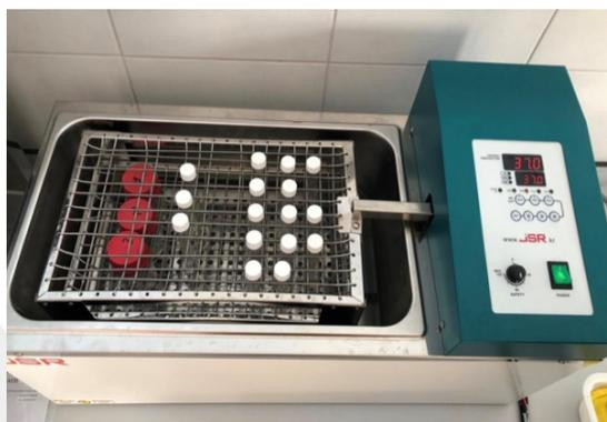
**Figure 3.3 :** Water shaking bath for degradation test of membranes.
